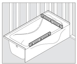
FIGURE 2. Check to assure tub is level.
